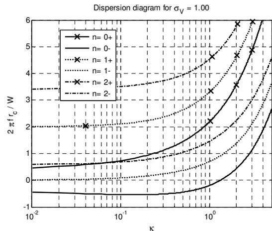
**Figure 2:** The dispersion diagram for a cavitating vortex
