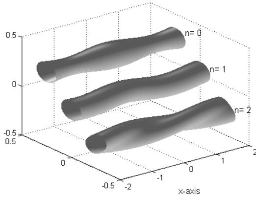
**Figure 1:** Visualisation of the spatial deformation of a cavitating vortex for the modes  $n=0, 1$  and  $2$  at one time-step.
