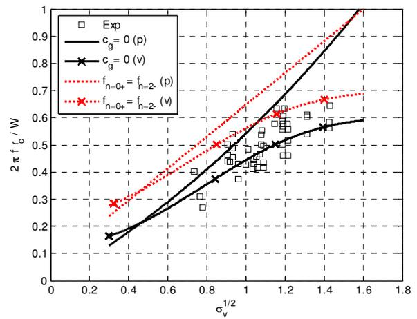
**Figure 4:** Comparison of the non-dimensional resonance frequency between the experimental data of Maines & Arndt [4], symbols, and theoretical curves for potential flow (p) and potential flow corrected for viscous effects (v). The theoretical curves are for zero group speed ( $c_g = 0$ ) and coinciding frequency.
