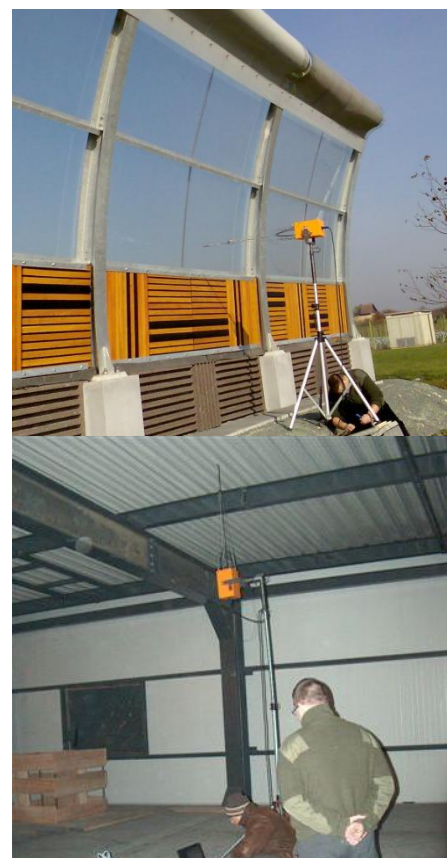
Figure 2: Typical application of the measuring system: upper picture – sample of a road noise barrier, lower picture – perforated sheet metal ceiling of an industrial hall.
