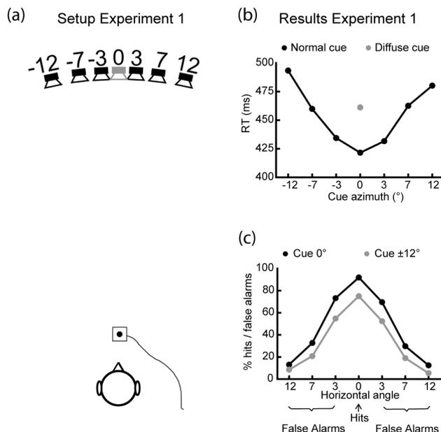
**Figure 1:** (a) Loudspeaker Set-up of Experiment 1. (b) The RT's measured in Experiment 1. (c) The percentage hits and false alarms obtained in Experiment 1.
