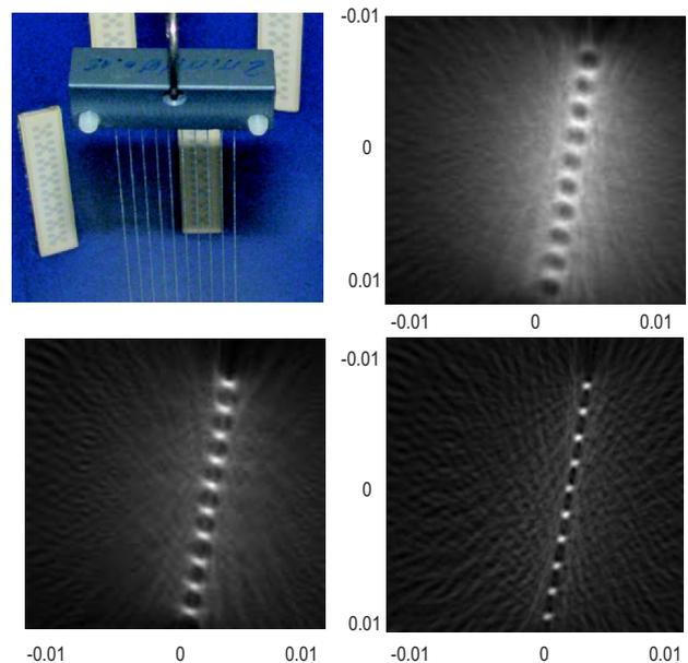
**Figure 2:** Top left: Experimental setup of ten nylon threads with diameter of 0.2 mm and distance of 2 mm. Top right to bottom left: Reconstructed images of coherent imaging with envelope, adapted matched filter, and adapted matched filter with Chirp excitation. Scaling in mm.
