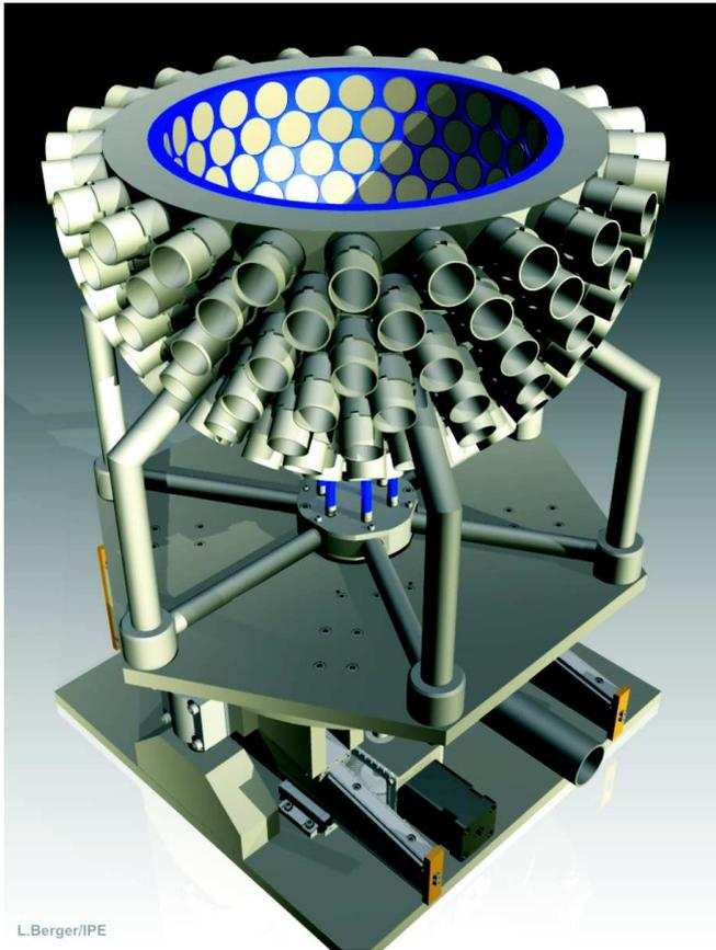
**Figure 3:** The image shows a technical drawing of the new semi-ellipsoidal aperture, new cylindrical TAS and the movement devices.
