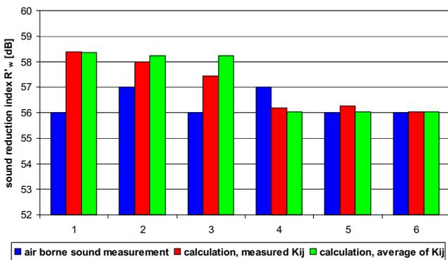
**Figure 6:** comparison between measured and calculated sound reduction index of **horizontal transmission** situations
