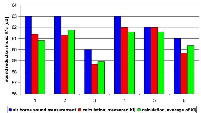
**Figure 5:** comparison between measured and calculated sound reduction index of vertical transmission situations
