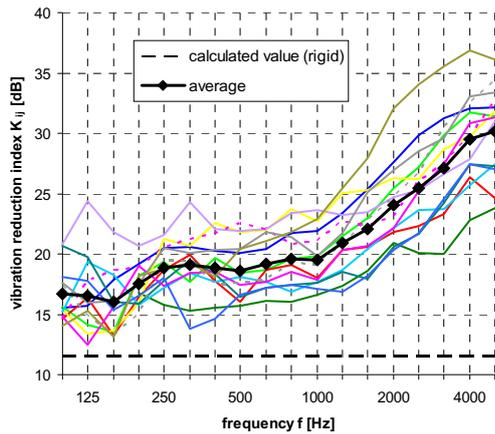
**Figure 3:** vibration reduction index  $K_{ij}$  of gypsum walls, measured in different buildings, path Df / Fd, vertical transmission
