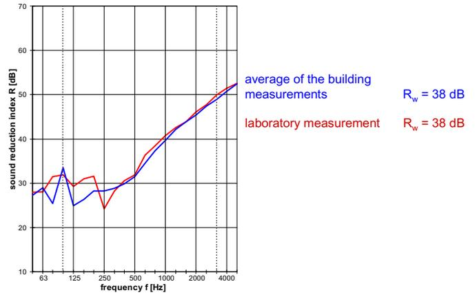
**Figure 2:** comparison of the sound reduction index, measured in the laboratory and in different buildings
