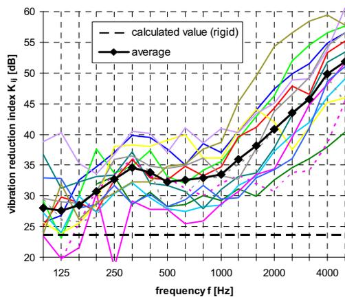
**Figure 4:** vibration reduction index  $K_{ij}$  of gypsum walls, measured in different buildings, path Ff, vertical transmission
