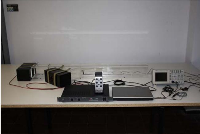
Figure 1: Rectangular duct in y-shape made from plexiglas with according signal processing (Pure Data), playback (4" mid-range transducer with amplifier), recording (electret condenser microphone capsules) and visualisation (oscilloscope) hardware.
