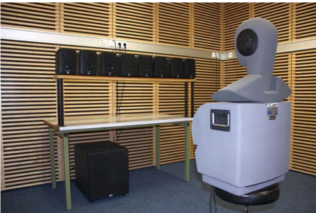
Figure 2: Stereo triangle configuration with a linear loudspeaker array of eight JBL Control 1 monitor loudspeaker and head and torso dummy from HEAD acoustics in our jury test room. Further necessary equipment, e. g. amplifier and RME Hammerfall audio interfaces is in the anteroom.
