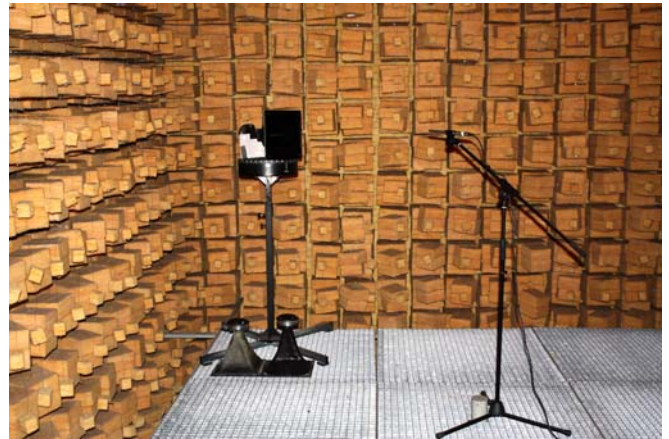
Figure 3: Experimental set-up consisting of B&C compression drivers with d&b horn prototypes, Outline ST 1 turntable and measuring microphone in our anechoic measuring room. This equipment is controlled by the D igital A udio A nalysis S oftware (DAAS) and Outline controller ET 1 which can be found in the side room.
