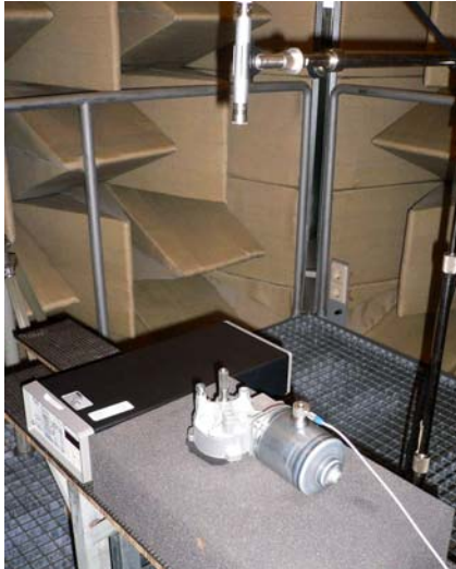
Figure 5: Airborne sound / solid-borne sound measurements (microphone / accelerometer) of electric motors from Nidec that have different implemented definite defects.
