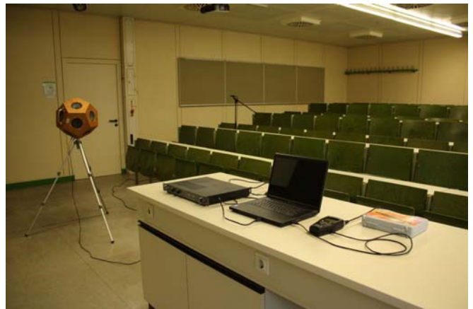
Figure 4: Dodecahedron with amplifier and appropriate portable measuring instrumentation (laptop, Acoustilyzer NTI AL1 with MiniSPL) for reverberation time measurements in different university-intern lecture rooms.
