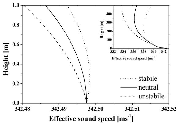
Figure 3: Mean urban profiles of the nighttime effective sound speed in upwind direction with temperature gradients:  $-0.01 \text{ Km}^{-1}$  (unstable),  $0 \text{ Km}^{-1}$  (neutral),  $+0.01 \text{ Km}^{-1}$  (stable).
