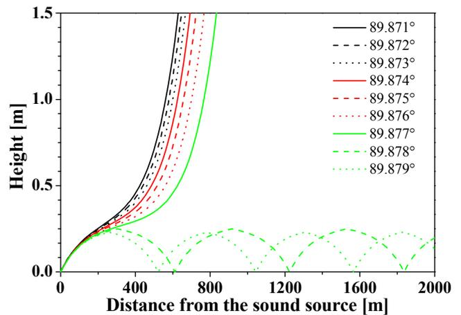
Figure 4: Sound rays with different emission angles during stable nighttime conditions (see Figure 3) in upwind direction.
