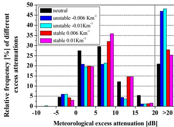
Figure 7: Relative frequency of different meteorological excess attenuations during nighttime conditions and several thermal stratifications (temperature gradients).
