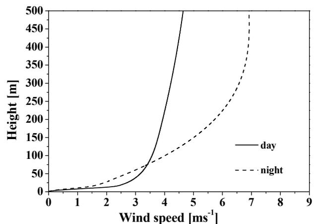
**Figure 1:** Mean urban wind speed profile daytime and nighttime. The roughness height was 1 m.
