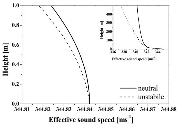
Figure 2: Mean urban profiles of the daytime effective sound speed in upwind direction with temperature gradients:  $-0.01 \text{ Km}^{-1}$  (unstable),  $0 \text{ Km}^{-1}$  (neutral).
