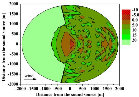
Figure 6: Meteorological excess attenuation [dB] during nighttime conditions and a stable stratification.
