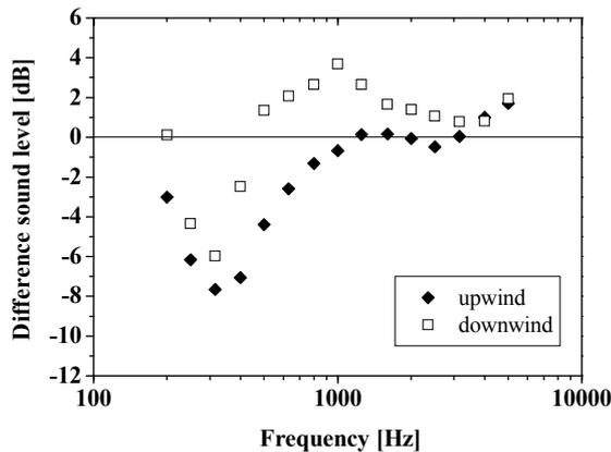
**Figure 8:** Difference sound level (60-min mean) from measurements and VDI model at a distance of 150 m from a highway with a noise barrier during daytime conditions in upwind and downwind direction.
