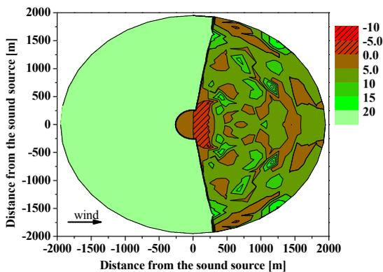
Figure 5: Meteorological excess attenuation [dB] during nighttime conditions and an unstable stratification.
