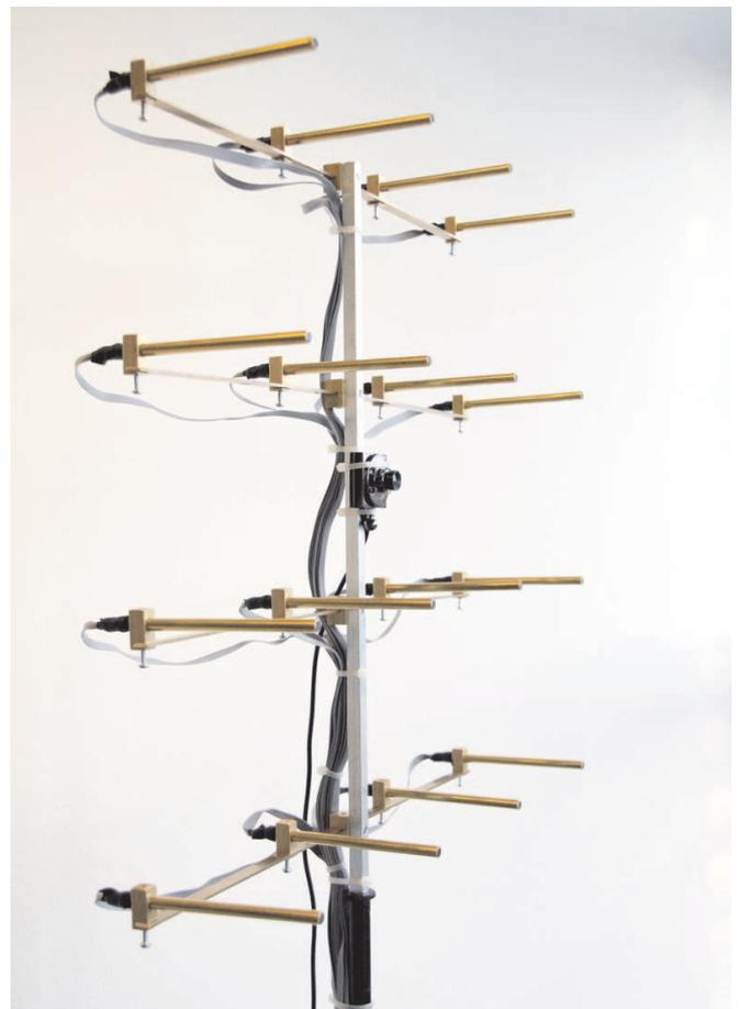
**Figure 3:** Four by four microphone test array with a camera in the center. The depicted microphone spacing is 15 cm.
