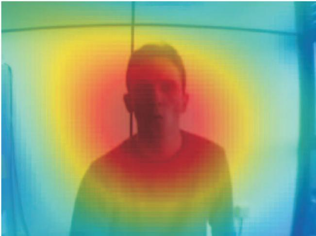
**Figure 4:** Beamforming demonstration: whistling at approximately one meter distance from the array. The red regions indicate large pressure signal amplitudes, the blue regions indicate small amplitudes.
