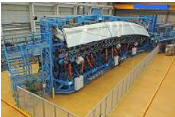
Figure 2: Hydraulic testing facility for airfoil wings.
