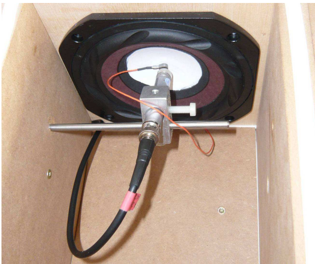
Figure 4: Arrangement of the accelerometer and microphone at the secondary source
