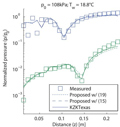
**Figure 1:** Comparison of recorded and simulated fundamental (top) and second harmonic (bottom) for a 5 cycle, 1 MHz sinusoidal burst during a propagation experiment at 108 kPa as a function of depth.
