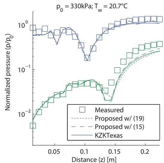
**Figure 2:** Comparison of recorded and simulated fundamental (top) and second harmonic (bottom) for a 5 cycle, 1 MHz sinusoidal burst during a propagation experiment at 330 kPa as a function of depth.
