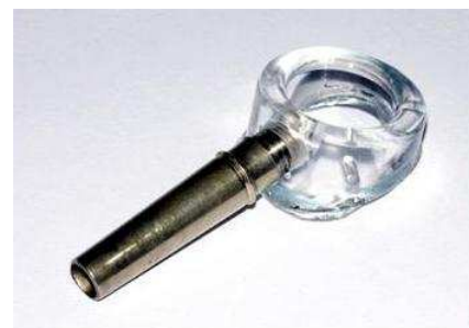
Figure 1: Perspex horn mouthpiece with optical glass window for visual access.
