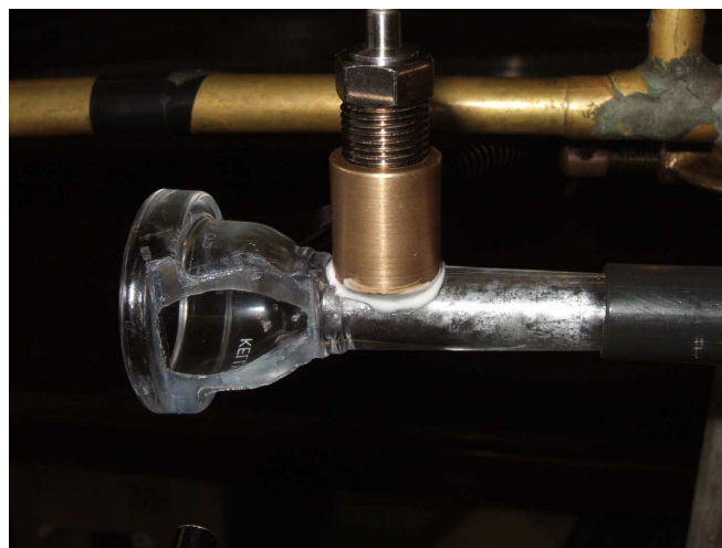
Figure 2: A photograph of the mouthpiece showing the window and PCB microphone adaptor
