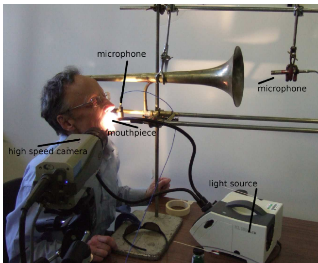
Figure 4: The complete experimental setup, showing the position of the mouthpiece, camera, and microphones. Measurements were taken on a tenor trombone, using three different musicians—amateurs with many years playing experience. Players were asked to sound notes of the same pitch but at varying dynamic level—the first at a mezzo forte ( mf ) level and the second as loudly as possible ( fff ). The radiated sound was recorded at a distance of one bell radius.
