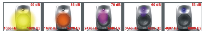
Figure 1: Multiband view of a two-way loudspeaker. Broadband noise with decreasing level to higher frequencies.
