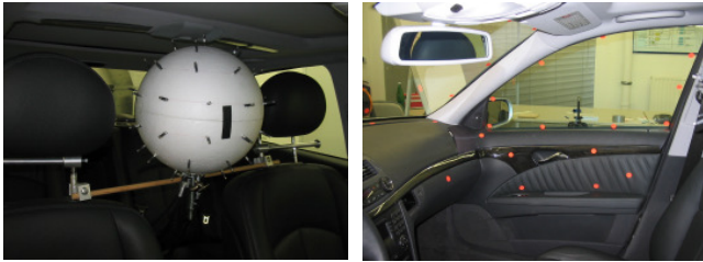
Figure 13: Beamforming with measured transfer functions. Array placed in the middle of the cabin (left). Speaker positions (red dots) for the measurement of the transfer functions (right).
