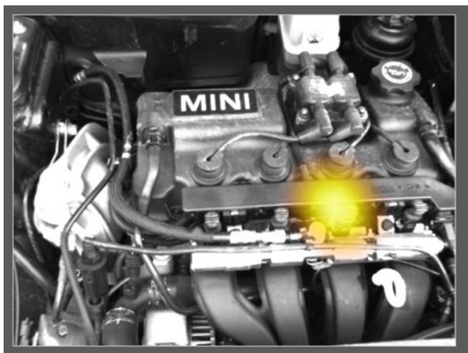
Figure 9: Noise radiation of the third cylinder in the 2-4 kHz frequency band.
