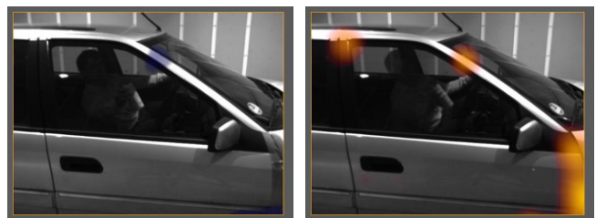
Figure 12: Leakage detection with compressed air. In case of a damaged inner sealing the noise is radiated at the damage point as well as on both ends of the sealing (right picture)
