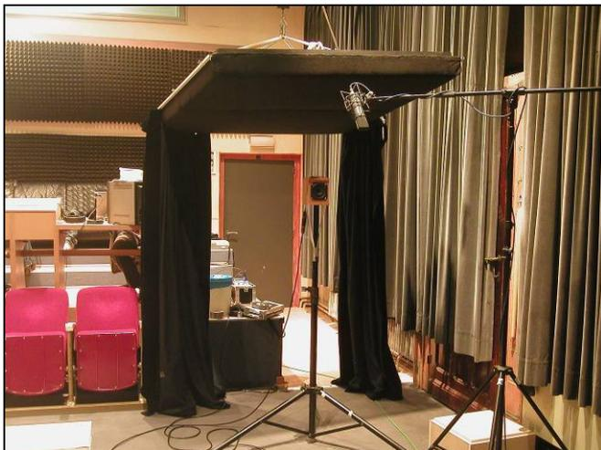
Figure 3: Typical Foley setup with tent (opened) and microphone
