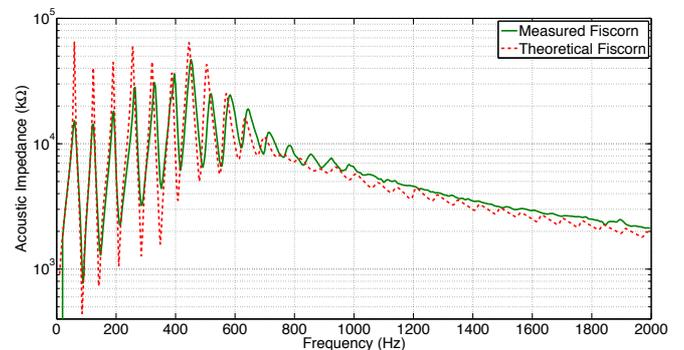
**Figure 1:** Input impedance curves measured for a 2.4m long fiscorn at playing conditions (*solid line*) and theoretically calculated (*dashed line*).
