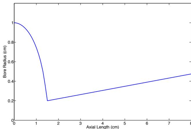
**Figure 3:** A plot of the internal bore profile for the lituus mouthpiece.
