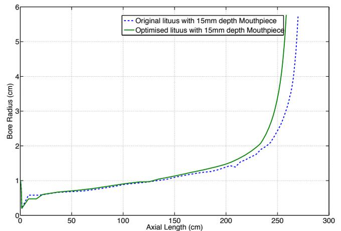
**Figure 4:** A plot of the internal bore profile for the unoptimised (*dashed line*) and optimised (*solid line*) lituus design.
