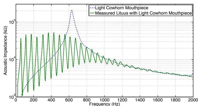
**Figure 7:** Input impedance curves measured for the constructed lituus (solid line) and the constructed lituus mouthpiece (dashed line).
