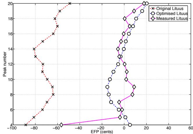
**Figure 6:** Plot of mode number versus Equivalent Fundamental Pitch (in cents) for the original lituus design, theoretical optimised lituus design, and the constructed lituus.
