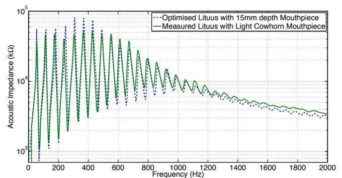
**Figure 5:** Input impedance curves measured for the constructed lituus (*solid line*) and theoretically calculated from the optimised design (*dashed line*).
