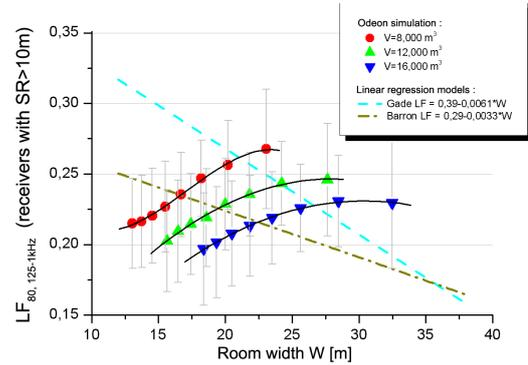
**Figure 3:** Relation between  $LF_{80}$  and room width shown for Odeon simulation and for two regression models (by Gade and Barron) grouped by models volume
