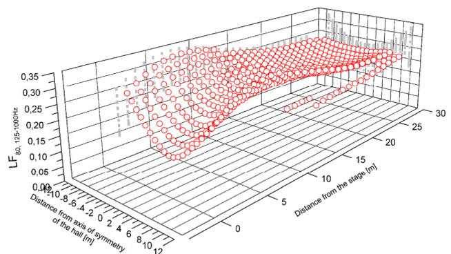
**Figure 8:** Typical “tongue-shape” distribution of Early Lateral Energy Fraction LF<sub>80, 250Hz</sub> in rectangular rooms (model 5, Volume 12,000 m<sup>3</sup>). Models n<sup>o</sup> – see Fig.1.
