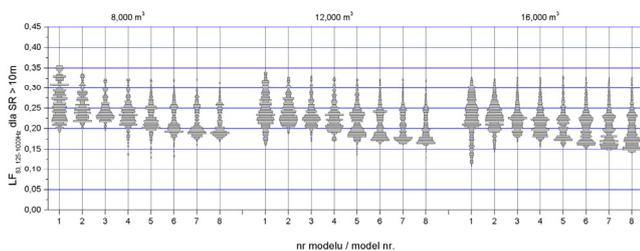
**Figure 5:** Histograms comparison of Early Lateral Energy Fraction LF<sub>80, 125-1kHz</sub>, calculated by Odeon (grid response) in all analyzed volumes and models. Models n<sup>o</sup> see Fig.1.
