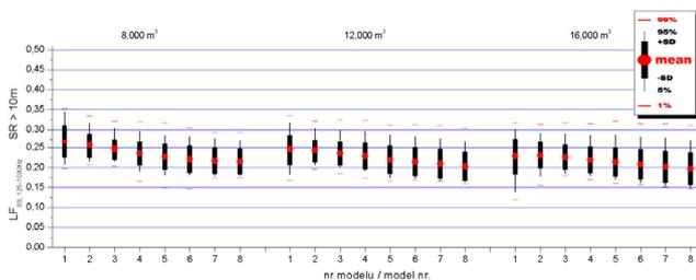
**Figure 2:** Comparison of room-averaged Early Lateral Energy Fraction  $LF_{80, 125-1kHz}$  calculated by Odeon (grid response) in all analyzed volumes and models. Models n° - see Fig.1
