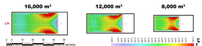
**Figure 7:** Comparison of distribution of Early Lateral Energy Fraction LF<sub>80, 250Hz</sub>, calculated by Odeon (grid response) in model 5 in all volumes. Models n<sup>o</sup> – see Fig.1.
