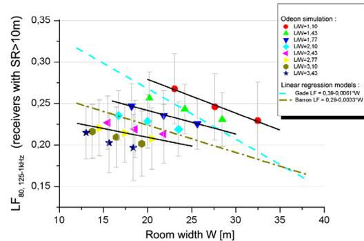
**Figure 4:** Relation between  $LF_{80}$  and room width shown for Odeon simulation and for two regression models (by Gade and Barron), grouped by models length-to-width ratio
