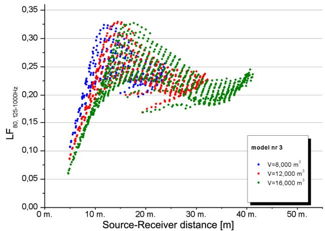
**Figure 6:** Relation of Early Lateral Energy Fraction LF<sub>80, 125-1kHz</sub> from Source-Receiver distance, for model 3 in all analyzed volumes (including receivers closer then 10m from source). Models n<sup>o</sup> – see Fig.1.
