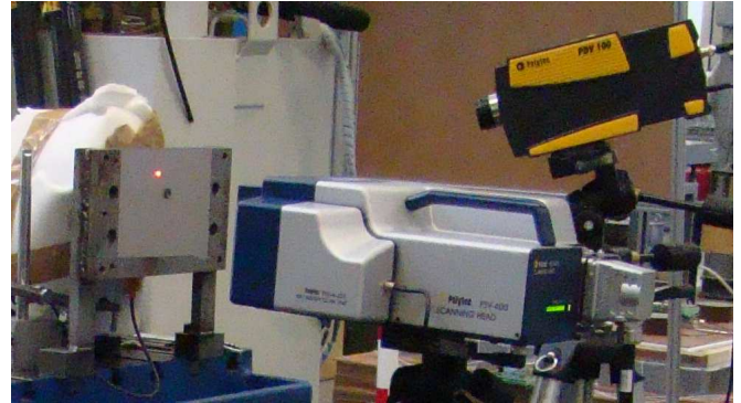
Figure 1: Measurement setup for the scanning laser Doppler vibrometer
