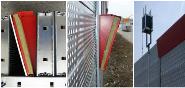
Figure 3: The added device tested during these measurements before mounting (left), after the mounting in the middle of the barrier (middle) and on the top of the barrier (right).
