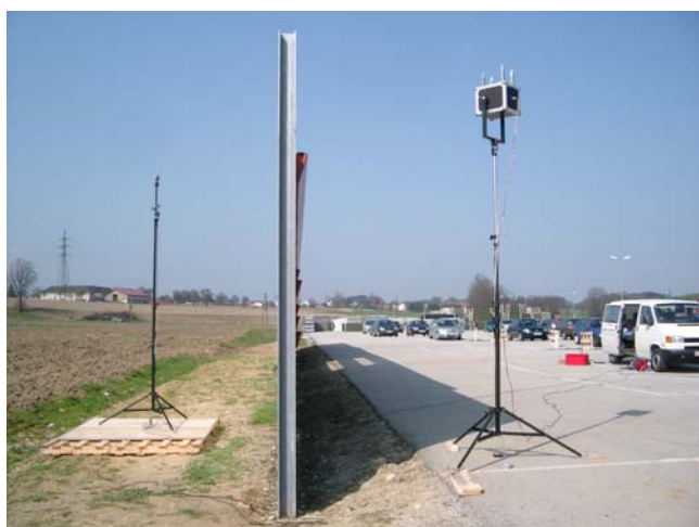
Figure 4: The setup of the measurements for sound diffraction for the source position S4 using an angle of 45° between the noise barrier and the line connecting source and microphones.
