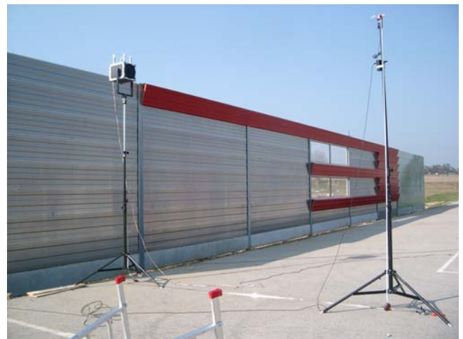
Figure 5: The setup for the free-field measurement for the source position S1 (using normal incidence).
