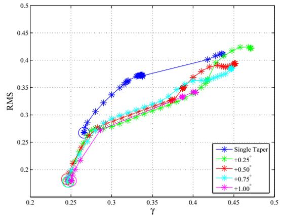
**Figure 4:** RMS amplitude of  $p$  (pressure inside the mouthpiece as solved by *harmbal*) vs  $\gamma$  for all five bore configurations
