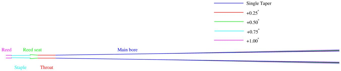
**Figure 1:** Schematic showing the bore profile of the five virtual instruments studied
