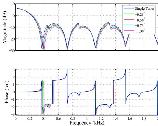
**Figure 6:** Calculated transfer function of the chanter for five bore configurations
