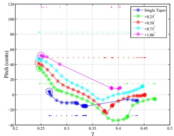
**Figure 5:** Pitch vs.  $\gamma$  for all five bore configurations. 0 cents corresponds to the frequency of the note  $F_4^\#$  (370 Hz). The horizontal dotted lines represent frequencies of the first air column resonance.
