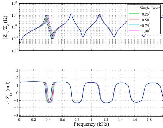
**Figure 3:** Calculated input impedance of the chanter
