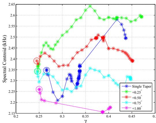
**Figure 7:** Spectral centroid vs.  $\gamma$  for all five bore configurations
