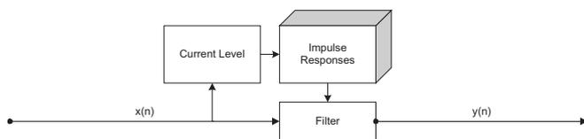
**Figure 3:** Model 1 - Block diagram of the model with nonlinear filtering with Look-Up-Table.
