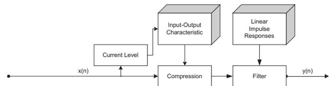
(a) Block diagram of the Hammerstein model with linear filtering and compression.
