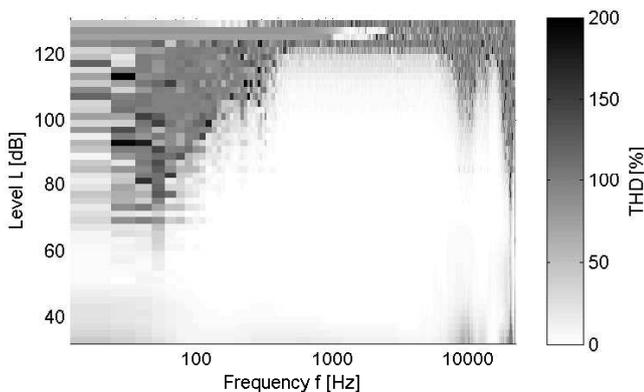
**Figure 1:** Total harmonic distortion of the hearing aid receiver in % plotted over the frequency  $f$  and the level  $L$ . The greynance is from 0% to 200%.
