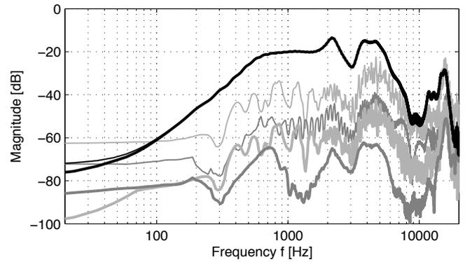
(a) Transfer function of the receiver for 120 dB SPL (thin lines) in comparison with the simulation of the model 1 - Nonlinear filtering with Look-Up-Table.
