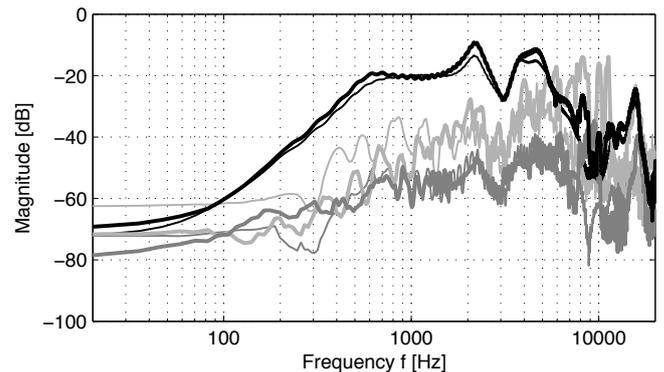
(c) Transfer function of the receiver for 120 dB SPL (thin lines) in comparison with the simulation of the model 3 - Nonlinear parallel filtering.
