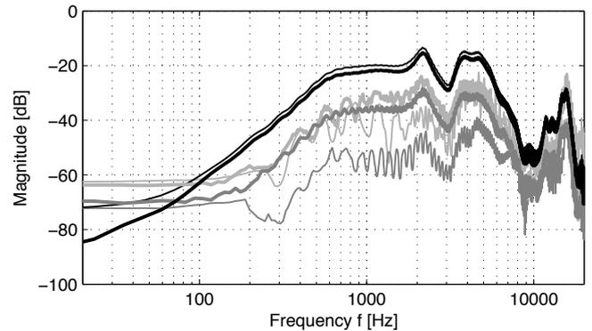
(b) Transfer function of the receiver for 120 dB SPL (thin lines) in comparison with the simulation of the model 2 - Hammerstein model with linear filtering and compression.
