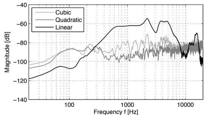
(c) Nonlinear transfer function of the receiver for 80 dB SPL.
