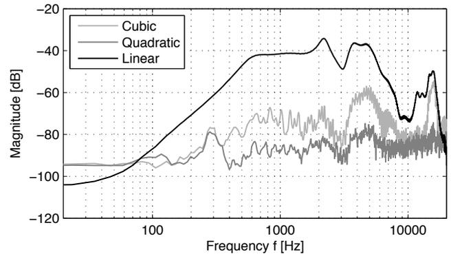
(b) Nonlinear transfer function of the receiver for 100 dB SPL.
