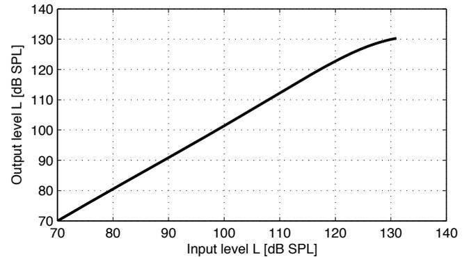
(b) Input-output characteristic of the receiver for  $f = 1$  kHz.
