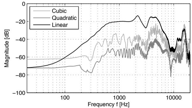
(a) Nonlinear Transfer functions of the receiver for 120 dB SPL.
