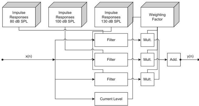
(a) Block diagram of the model with nonlinear parallel filtering.
