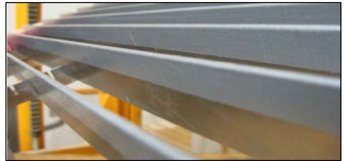
Figure 8: Bearing bars with tape-rounded edges
