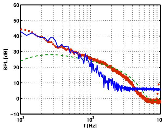
**Figure 6:** Comparison of sound measurements with numerical predictions using Curle's analogy and Amiet's theory.
