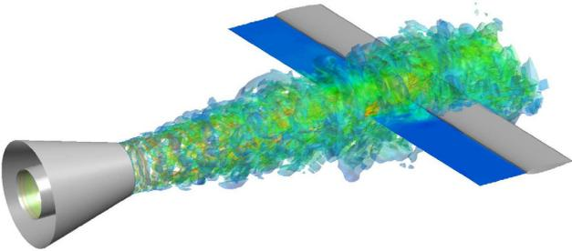
**Figure 3:** Instantaneous flow field around the airfoil, and spatial correlation extraction plane.
