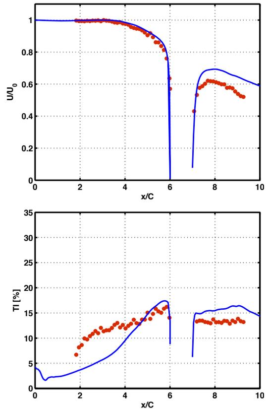
**Figure 4:** Comparison of experimental measurements with numerical computations : mean velocity profiles (up) and turbulence intensity profiles (bottom) along the  $x$ -axis.
