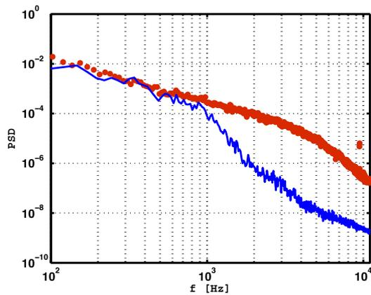
**Figure 5:** Comparison of experimental measurements with numerical computations : Power Spectrum Density of velocity magnitude fluctuations at  $(x, y) = (5D, 0)$  (bottom).
