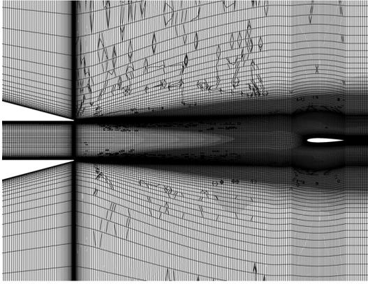
**Figure 2:** Mesh cells repartition in the  $x - z$  plane.
