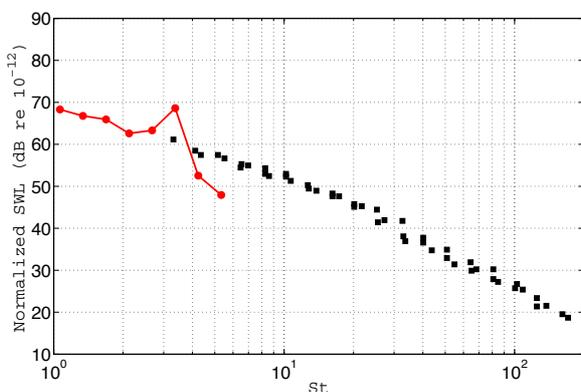
**Figure 2:** Comparison of the numerical simulations and the experimental study by Nelson and Morfey [1]. Nelson and Morfey's experiments (■), Numerical simulation (line).
