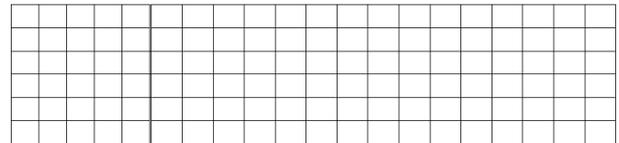
(c) Coarser target 500 elements meshes.
