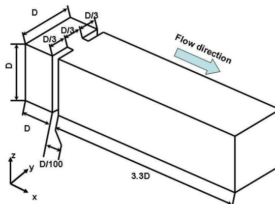
Figure 1: Diaphragm geometry.  $D = 0.3$  m.
