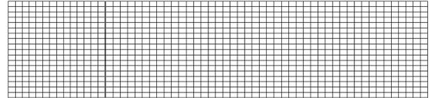
(b) Coarser target 5,000 elements mesh).
