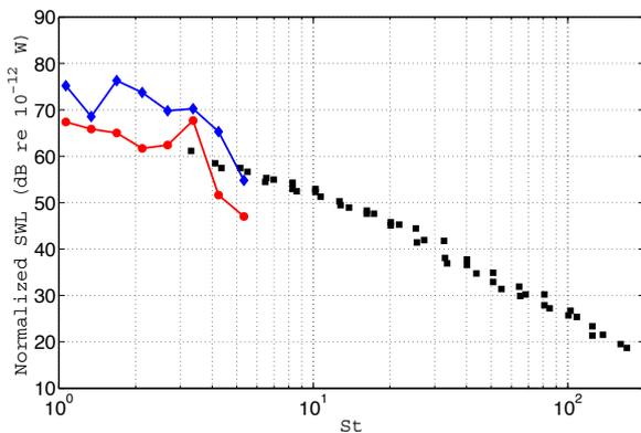
**Figure 5:** Comparison of the numerical simulations, the experimental study led by Nelson and Morfey [1] and the condensation of dipoles. Nelson and Morfey's experiments (■), Numerical simulation with dipoles field (●), Numerical simulation with equivalent dipole (◆).
