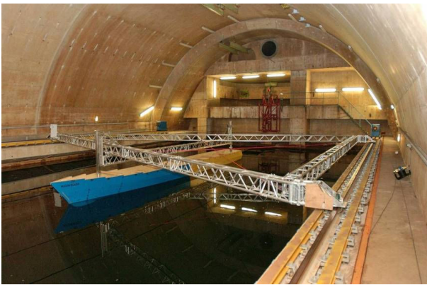
Figure 2: The specially developed 'silent towing system' in the towing tank of MARIN at Ede.
