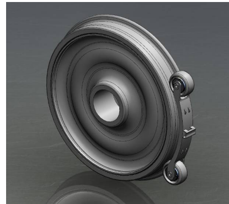
Figure 4: CAD-drawing of the roller applied on a wheel
