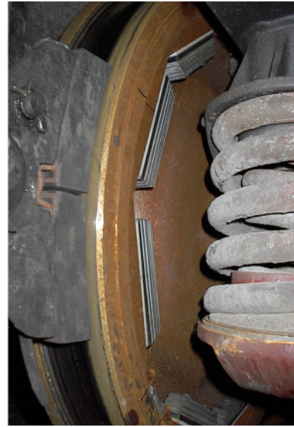
Figure 3: Recent wheel damper of the company Schrey & Veit to be improved within the project ‘LZarG’.
